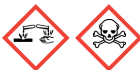
GHS05 Corrosion GHS06 Skull and crossbones
